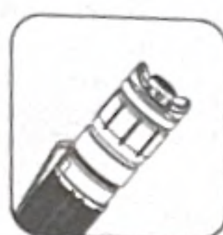
③ Screw the tail cap on tightly
