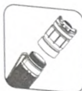
① Unscrew the tail cap
