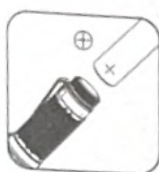
② Insert the battery with the positive terminal facing the flashlight head
